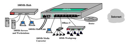
Figure 2.4e: The Magnum 528F provides a 100Mb port for backbone connection.
